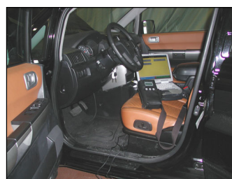
<Connecting the Measurement Adapter and Measurement Probe >
